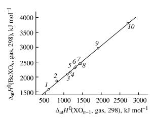
Atomization enthalpies of gaseous beryllium salts vs. atomization enthalpies of gaseous anion-forming oxides. (1) BePO<sub>2</sub>, (2) BeBO<sub>2</sub>, (3) BePO<sub>3</sub>, (4) BeMoO<sub>3</sub>, (5) BeWO<sub>3</sub>, (6) BeMoO<sub>4</sub>, (7) BeWO<sub>4</sub>, (8) and BeB<sub>2</sub>O<sub>4</sub>.
